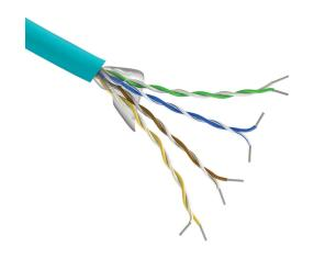
Quabbin continuous flexing Cat5e industrial Ethernet cable, unshielded, 4 twisted pairs, 24 AWG, 7/32-stranded, tinned copper, HDPE conductor insulation material, FR-TPE jacket, teal, cut to length.
