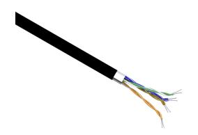
Quabbin Datamax Cat5e industrial Ethernet cable, shielded, 4 twisted pairs, 26 AWG, 7-stranded, tinned copper, polyolefin conductor insulation material, polyurethane jacket, black, cut to length.
