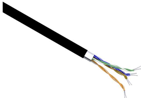
Quabbin Datamax Cat5e industrial Ethernet cable, shielded, 4 twisted pairs, 26 AWG, 7-stranded, tinned copper, polyolefin conductor insulation material, polyurethane jacket, black, cut to length.
