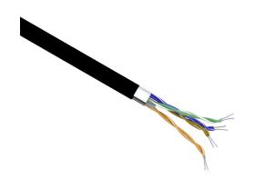
Quabbin Datamax continuous flexing Cat6a industrial Ethernet cable, shielded, 4 twisted pairs, 26 AWG, 7-stranded, tinned copper, HDPE conductor insulation material, Zero Halogen Flame Retardant (ZHFR) jacket, black, cut to length.
