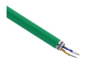
Quabbin continuous flexing Profinet cable, shielded, PLTC-ER and CM, 4 conductors, 22 AWG, tinned copper, polyethylene conductor insulation material, white, blue, yellow and orange, TPE jacket, green, cut to length.
