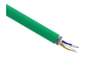
Quabbin continuous flexing Profinet cable, shielded, PLTC and CL3, 4 conductors, 22 AWG, tinned copper, polyethylene conductor insulation material, white, blue, yellow and orange, TPE jacket, green, cut to length.
