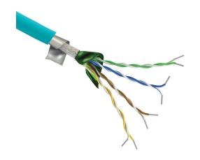
Quabbin continuous flexing Cat5e industrial Ethernet cable, shielded, 4 twisted pairs, 24 AWG, 7/32-stranded, tinned copper, HDPE conductor insulation material, FR-TPE jacket, teal, cut to length.
