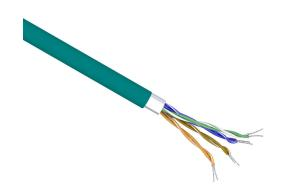
Quabbin Datamax continuous flexing Cat5e industrial Ethernet cable, shielded, 4 twisted pairs, 26 AWG, 7-stranded, tinned copper, HDPE conductor insulation material, TPE jacket, teal, cut to length.
