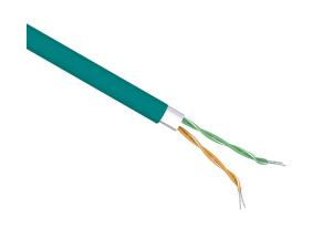
Quabbin Datamax continuous flexing Cat5e industrial Ethernet cable, shielded, 2 twisted pairs, 26 AWG, 7-stranded, tinned copper, HDPE conductor insulation material, Zero Halogen Flame Retardant (ZHFR) jacket, teal, cut to length.
