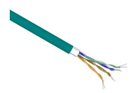
Quabbin Datamax continuous flexing Cat5e industrial Ethernet cable, shielded, 4 twisted pairs, 26 AWG, 7-stranded, tinned copper, HDPE conductor insulation material, Zero Halogen Flame Retardant (ZHFR) jacket, teal, cut to length.
