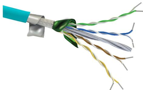
Quabbin continuous flexing Cat6/6a industrial Ethernet cable, shielded, 4 twisted pairs, 26 AWG, 7-stranded, tinned copper, polyethylene conductor insulation material, TPE jacket, teal, cut to length.
