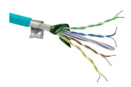
Quabbin continuous flexing Cat6/6a industrial Ethernet cable, shielded, 4 twisted pairs, 26 AWG, 7-stranded, tinned copper, polyethylene conductor insulation material, TPE jacket, teal, cut to length.
