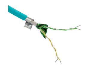
Quabbin continuous flexing Cat5e industrial Ethernet cable, shielded, 2 twisted pairs, 24 AWG, 7/32-stranded, tinned copper, HDPE conductor insulation material, FR-TPE jacket, teal, cut to length.
