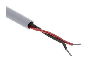
Quabbin control and signal cable, unshielded, 2 conductors, 18 AWG, 16-stranded, tinned copper, PVC conductor insulation material, PVC jacket, gray, cut to length.
