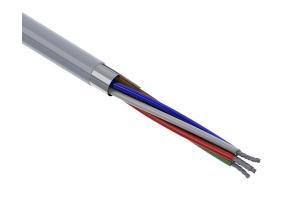
Quabbin control and signal cable, shielded, 6 conductors, 18 AWG, 16-stranded, tinned copper, PVC conductor insulation material, PVC jacket, gray, cut to length.
