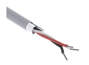
Quabbin control and signal cable, shielded, 3 conductors, 18 AWG, 16-stranded, tinned copper, PVC conductor insulation material, PVC jacket, gray, cut to length.
