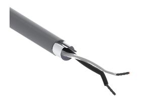
Quabbin control and signal cable, shielded, 2 conductors, 18 AWG, 16-stranded, tinned copper, PVC conductor insulation material, PVC jacket, gray, cut to length.
