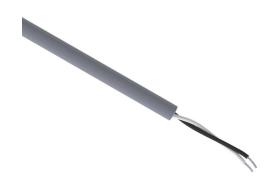
Quabbin control and signal cable, unshielded, 2 conductors, 18 AWG, 7-stranded, tinned copper, PVC conductor insulation material, PVC jacket, gray, cut to length.
