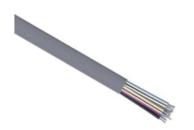
Quabbin control and signal cable, unshielded, 25 conductors, 18 AWG, 16-stranded, tinned copper, PVC conductor insulation material, PVC jacket, gray, cut to length.
