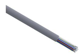
Quabbin control and signal cable, unshielded, 19 conductors, 18 AWG, 16-stranded, tinned copper, PVC conductor insulation material, PVC jacket, gray, cut to length.
