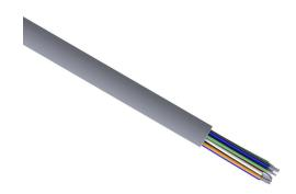
Quabbin control and signal cable, unshielded, 15 conductors, 18 AWG, 16-stranded, tinned copper, PVC conductor insulation material, PVC jacket, gray, cut to length.
