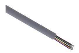
Quabbin control and signal cable, unshielded, 12 conductors, 18 AWG, 16-stranded, tinned copper, PVC conductor insulation material, PVC jacket, gray, cut to length.
