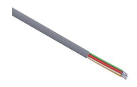
Quabbin control and signal cable, unshielded, 7 conductors, 18 AWG, 16-stranded, tinned copper, PVC conductor insulation material, PVC jacket, gray, cut to length.
