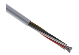
Quabbin control and signal cable, unshielded, 5 conductors, 18 AWG, 16-stranded, tinned copper, PVC conductor insulation material, PVC jacket, gray, cut to length.
