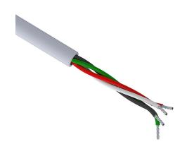
Quabbin control and signal cable, unshielded, 4 conductors, 18 AWG, 16-stranded, tinned copper, PVC conductor insulation material, PVC jacket, gray, cut to length.
