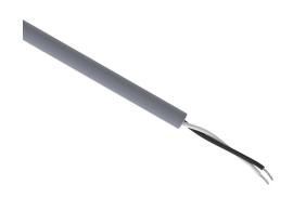
Quabbin control and signal cable, unshielded, 2 conductors, 16 AWG, 19-stranded, tinned copper, PVC conductor insulation material, PVC jacket, gray, cut to length.
