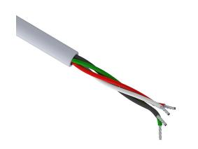
Quabbin control and signal cable, unshielded, 4 conductors, 16 AWG, 19-stranded, tinned copper, PVC conductor insulation material, PVC jacket, gray, cut to length.
