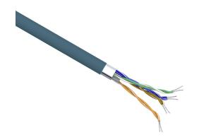
Quabbin Datamax Cat6a Ethernet cable, shielded, 4 twisted pairs, 26 AWG, 7-stranded, tinned copper, polyethylene conductor insulation material, PVC jacket, blue, cut to length.
