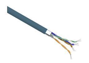
Quabbin Datamax Cat6 Ethernet cable, shielded, 4 twisted pairs, 26 AWG, 7-stranded, tinned copper, polyethylene conductor insulation material, PVC jacket, blue, cut to length.
