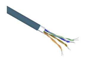
Quabbin Datamax Cat5e Ethernet cable, shielded, 4 twisted pairs, 26 AWG, 7-stranded, tinned copper, polyethylene conductor insulation material, PVC jacket, blue, cut to length.
