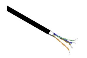
Quabbin Datamax Cat6a Ethernet cable, shielded, 4 twisted pairs, 26 AWG, 7-stranded, tinned copper, HDPE conductor insulation material, low smoke zero halogen (LSZH) jacket, black, cut to length.
