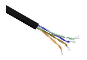
Quabbin Datamax Cat6 Ethernet cable, unshielded, 4 twisted pairs, 28 AWG, 7-stranded, tinned copper, HDPE conductor insulation material, low smoke zero halogen (LSZH) jacket, black, cut to length.
