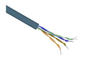
Quabbin Datamax Cat6e Ethernet cable, unshielded, 4 twisted pairs, 24 AWG, 7-stranded, tinned copper, polyethylene conductor insulation material, PVC jacket, blue, cut to length.
