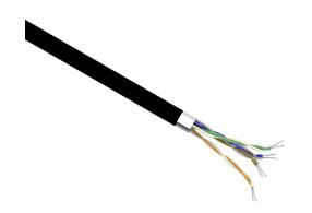
Quabbin Datamax Cat6 Ethernet cable, shielded, 4 twisted pairs, 26 AWG, 7-stranded, tinned copper, foamed FEP conductor insulation material, PVC jacket, black, cut to length.
