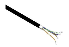
Quabbin Datamax Cat6a Ethernet cable, shielded, 4 twisted pairs, 26 AWG, 7-stranded, tinned copper, foamed FEP conductor insulation material, PVC jacket, black, cut to length.
