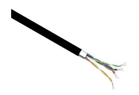
Quabbin Datamax Cat6 Ethernet cable, shielded, 4 twisted pairs, 28 AWG, 7-stranded, tinned copper, foamed FEP conductor insulation material, PVC jacket, black, cut to length.
