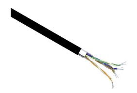
Quabbin Datamax Cat6a Ethernet cable, shielded, 4 twisted pairs, 28 AWG, 7-stranded, tinned copper, foamed FEP conductor insulation material, PVC jacket, black, cut to length.
