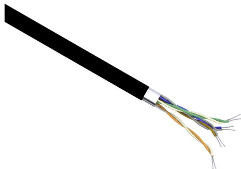
Quabbin Datamax Cat6a Ethernet cable, shielded, 4 twisted pairs, 28 AWG, 7-stranded, tinned copper, foamed FEP conductor insulation material, PVC jacket, black, cut to length.
