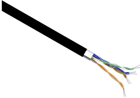
Quabbin Datamax Cat6 Ethernet cable, shielded, 4 twisted pairs, 26 AWG, 7-stranded, tinned copper, HDPE conductor insulation material, low smoke zero halogen (LSZH) jacket, black, cut to length.
