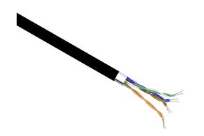
Quabbin Datamax Cat6 Ethernet cable, shielded, 4 twisted pairs, 26 AWG, 7-stranded, tinned copper, HDPE conductor insulation material, low smoke zero halogen (LSZH) jacket, black, cut to length.
