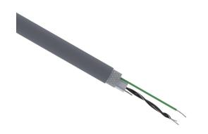
Quabbin RS-422/RS-485 low capacitance data serial cable, shielded, 1.5 twisted pair (includes ground), 20 AWG, 7-stranded, tinned copper, polyethylene conductor insulation material, PVC jacket, gray, cut to length.
