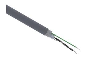
Quabbin RS-422/RS-485 low capacitance data serial cable, shielded, 1.5 twisted pair (includes ground), 20 AWG, 7-stranded, tinned copper, polyethylene conductor insulation material, PVC jacket, gray, cut to length.
