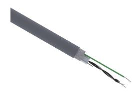
Quabbin RS-422/RS-485 low capacitance data serial cable, shielded, 1.5 twisted pair (includes ground), 22 AWG, 7-stranded, tinned copper, polyethylene conductor insulation material, PVC jacket, gray, cut to length.
