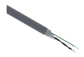
Quabbin RS-422/RS-485 low capacitance data serial cable, shielded, 1.5 twisted pair (includes ground), 24 AWG, 7-stranded, tinned copper, polyethylene conductor insulation material, PVC jacket, gray, cut to length.
