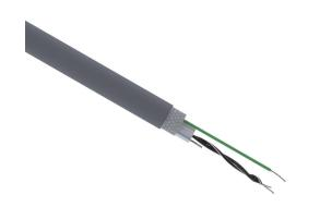
Quabbin RS-422/RS-485 low capacitance data serial cable, shielded, 1.5 twisted pair (includes ground), 24 AWG, 7-stranded, tinned copper, polyethylene conductor insulation material, PVC jacket, gray, cut to length.
