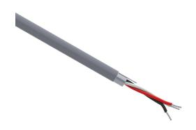
Quabbin control and signal cable, shielded, 1 twisted triad, 18 AWG, 16-stranded, tinned copper, PVC conductor insulation material, PVC jacket, gray, cut to length.
