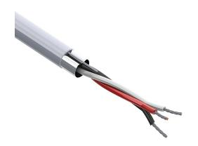
Quabbin control and signal cable, shielded, 3 conductors, 20 AWG, 10-stranded, tinned copper, PVC conductor insulation material, PVC jacket, gray, cut to length.
