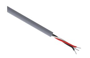
Quabbin control and signal cable, unshielded, 3 conductors, 18 AWG, 16-stranded, tinned copper, PVC conductor insulation material, PVC jacket, gray, cut to length.
