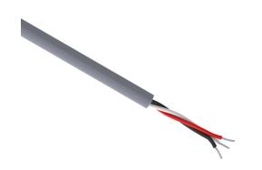
Quabbin control and signal cable, unshielded, 3 conductors, 20 AWG, 10-stranded, tinned copper, PVC conductor insulation material, PVC jacket, gray, cut to length.
