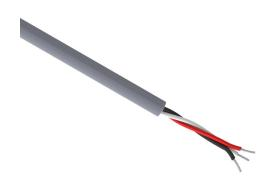
Quabbin control and signal cable, unshielded, 3 conductors, 22 AWG, 7-stranded, tinned copper, PVC conductor insulation material, PVC jacket, gray, cut to length.
