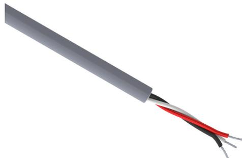
Quabbin control and signal cable, unshielded, 3 conductors, 22 AWG, 7-stranded, tinned copper, PVC conductor insulation material, PVC jacket, gray, cut to length.
