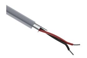
Quabbin control and signal cable, shielded, 1 twisted pair, 18 AWG, 16-stranded, tinned copper, PVC conductor insulation material, PVC jacket, gray, cut to length.
