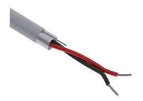
Quabbin control and signal cable, shielded, 2 conductors, 20 AWG, 10-stranded, tinned copper, PVC conductor insulation material, PVC jacket, gray, cut to length.
