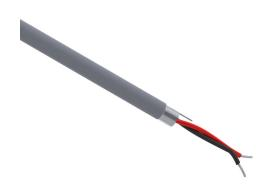
Quabbin control and signal cable, shielded, 2 conductors, 22 AWG, 7-stranded, tinned copper, PVC conductor insulation material, PVC jacket, gray, cut to length.
