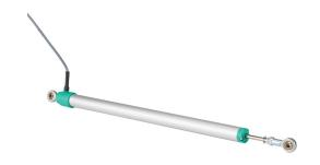
Gefran potentiometer linear position sensor, pivoting slide, 250mm stroke, 19mm diameter x 385mm body, rod eyes mount, pigtail, 3.2ft/1m cable length.
