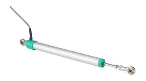
Gefran potentiometer linear position sensor, pivoting slide, 150mm stroke, 19mm diameter x 235mm body, rod eyes mount, pigtail, 3.2ft/1m cable length.
