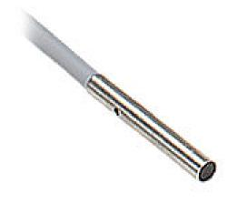
AutomationDirect inductive proximity sensor, tubular, 3mm diameter x 22mm body, stainless steel housing, NPN, N.O. output, 1mm sensing distance, flush, 3 kHz switching frequency, IP67, pigtail.
